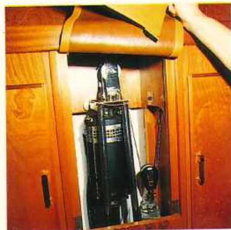
Left, well designed head with deep sink and cave lockers. Above, electric bow thruster retracted in a forepeak locker
