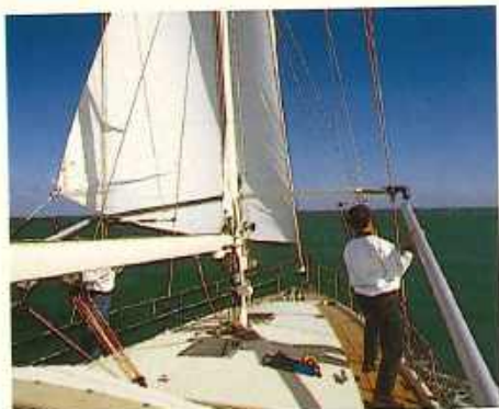
The running pole is rigged on the side deck and the sheet rove through the end fitting before being swung forward
