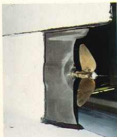
Transmission leg in position with propeller fitted and the wing keel ready for finishing
