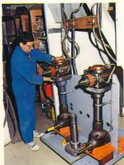
Custom-built transmission leg being bench-tested before installation
